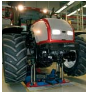
Testing system for tractors and PDA equipment user interface functioning as test monitor at the Valtra Oy Ab Suolahti factory
